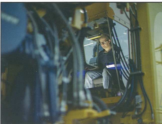
Fig. 3: Fully enclosed and insulated work cabin of the UNIMAT 09-4x4/4S E 3 (Photo: Plasser & Theurer)
