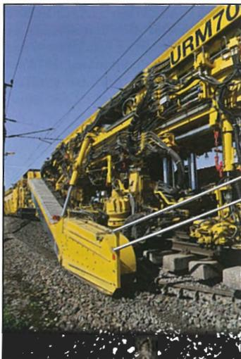
The shoulder ballast excavation unit excavates the shoulder ballast on the free side of the track and transfers it to the ballast screening unit. The free space thus created allows the slewable ballast excavation chain to be easily inserted underneath the track panel – no track panel dismantling or access hole digging is required;
