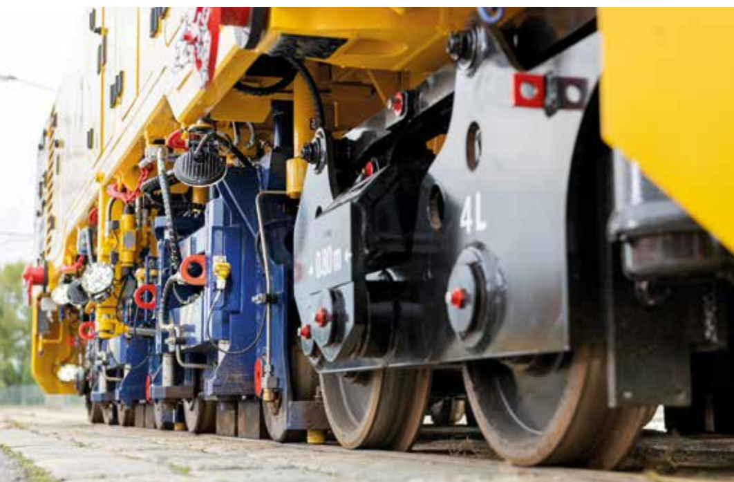
Fig 3. The grinding units of the ATMO oscillating rail grinder have been configured to cope with tight curve radii.
