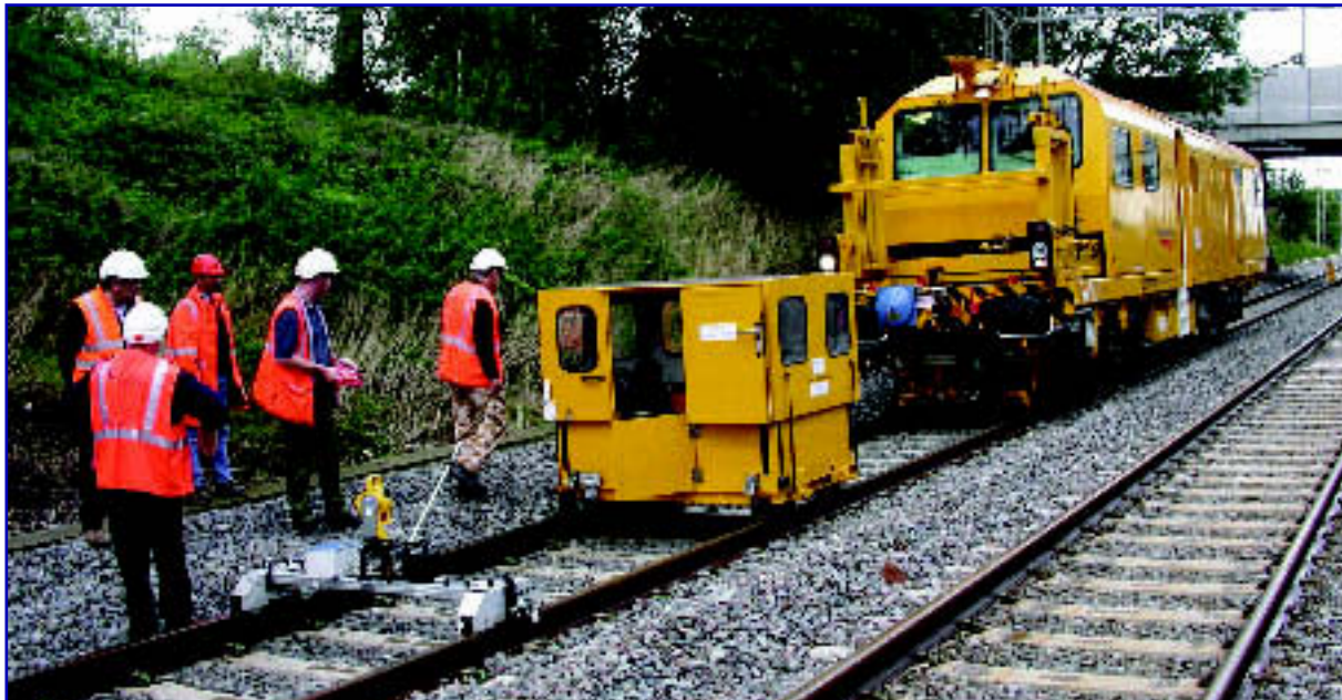
Figure 3: Network Rail's Automatic Track Geometry Survey Machine EM-SAT
