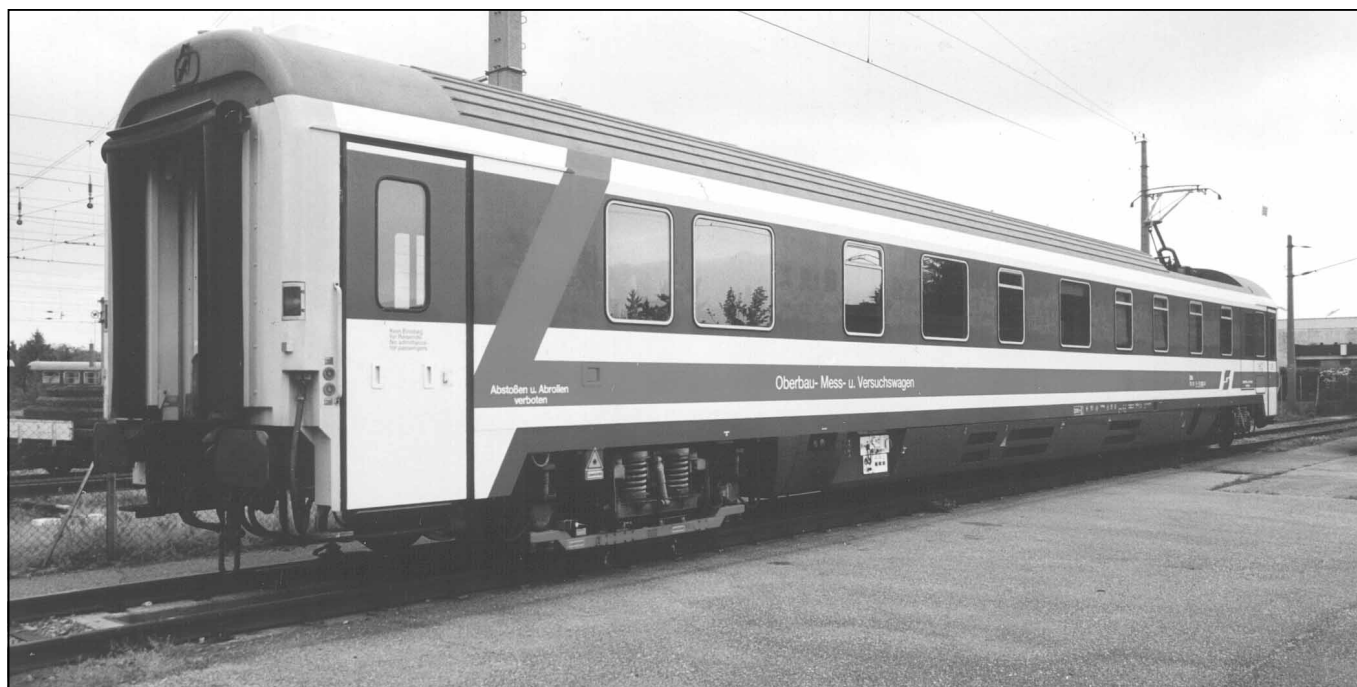
Fig. 1: Plasser & Theurer EM 250 high-speed track recording coach
