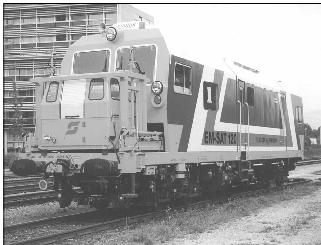
Fig. 3: Plasser & Theurer EM-SAT 120 track survey car
