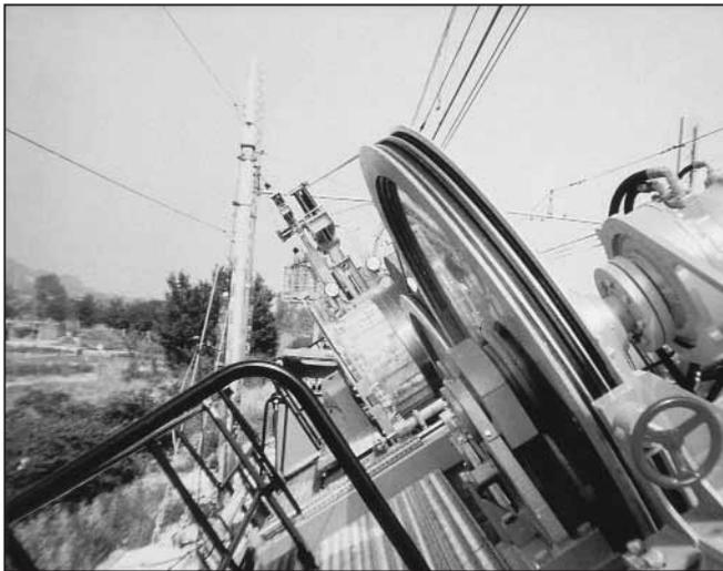
Fig. 3: Winch unit in tilted position
