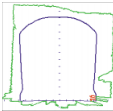
Fig 3. TunnelClient in standard mode. The current header, location and track geometry parameters are shown, with the actual measured data and the corresponding clearance diagram. The measured data violates the clearance in the lower right corner, and therefore this part of the profile is shown in red. As this profile is of a curve, the clearance diagram is enlarged on both sides to adjust for radius and superelevation
