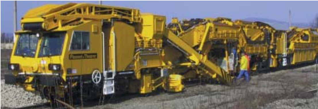
Figure 12: RM 95 RT ballast cleaning machine according to standards developed for British Rail
