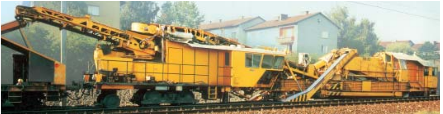
Figure 3: RM 80 U ballast cleaning machine
