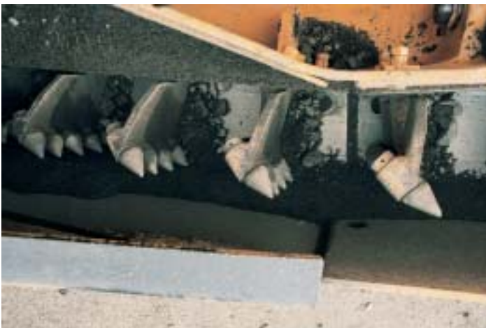
Figure 4: Excavating chain – scraper shovels with 4 fingers
