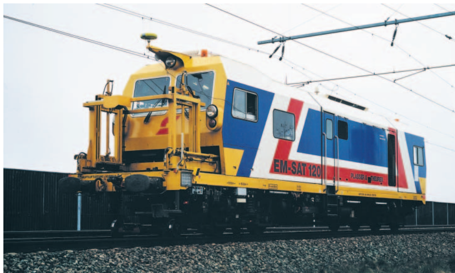
Fig. 1: Recording car with lifting device for the SAT
