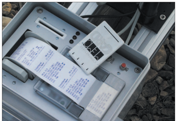
Fig. 3a: Storage card at the fixed point measuring unit
